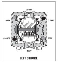
FIGURE 3 At completion of the stroke, the air valve again redirects air to the back side diaphragm A, which starts diaphragm B of on its exhaust stroke. As the pump reaches its original starting point, each diaphragm has gone through one exhaust and one discharge stroke. This constitutes one complete pumping cycle. The pump may prime take several cycles to completely depending on the conditions of the application
